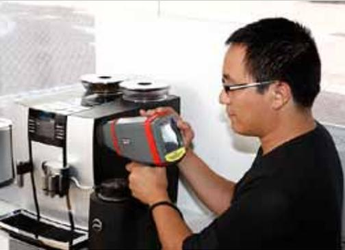
**THIS HANDHELD ENERGY DISPERSIVE X-RAY FLUORESCENCE (EDXRF) SPECTROMETER** has exceptional performance for this class of instrument, and can provide laboratory quality screening results in a matter of seconds. The SPECTRO xSORT has been optimized for fatigue-free on-site measurements.
