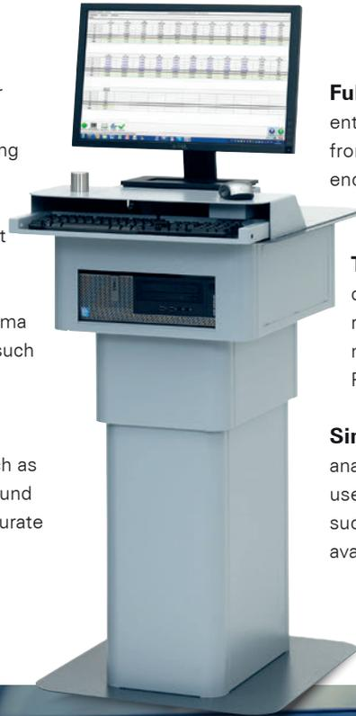
**Full spectrum scan.** Captures full coverage of entire relevant analytical spectrum simultaneously, from 120 to 770 nm. So allows comparison of encountered spectra to investigate elements not installed or expected.
