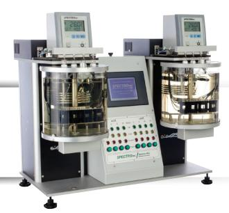
The SpectroVISC Q310 is a self-contained, bench-top automatic kinematic temperature dual bath viscosity measuring system that is ideal for in-service oil analysis laboratories that need to test a wide range of lubricant viscosities in a relatively short analysis cycle. The system conforms to the precise requirements of ASTM D445, D446, D7279, IP 71, ISO 3104 and ASTM D2270 for calculating viscosity index.
