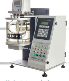
The SpectroVISC 0300 is a bench-top semi-automatic kinematic temperature bath viscometer optimized for the analysis of used and new lubricants. It conforms to the requirements in ASTM D445, D446, D7279, IP 71 and ISO 3104. It is also the ideal system for used oil analysis laboratories that need to test a wide range of lubricant viscosities.
