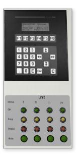
The SpectroVISC 0300 can be operated from the built-in control panel or from an optional external PC.
