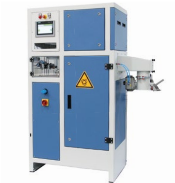
HTS 3000 cup wheel grinder
