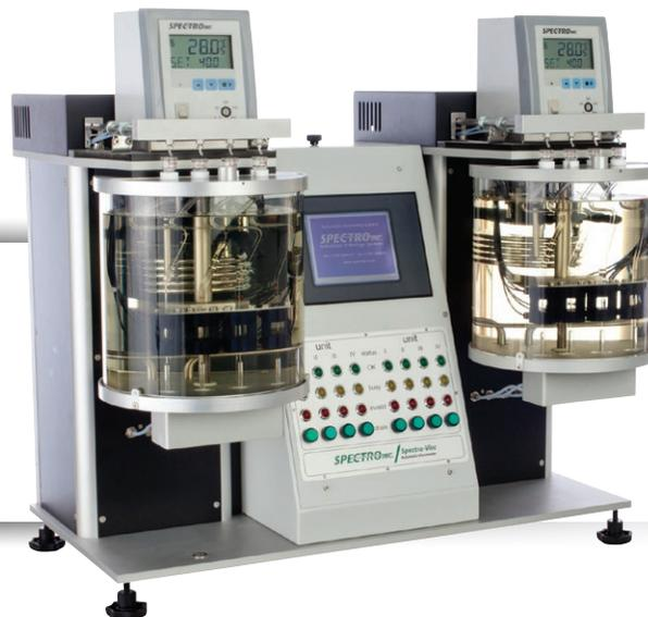
The SpectroVISC Q310 is a self-contained, bench-top automatic kinematic temperature dual bath viscosity measuring system that is ideal for in-service oil analysis laboratories that need to test a wide range of lubricant viscosities in a relatively short analysis cycle. The system conforms to the precise requirements of ASTM D445, D446, D7279, IP 71, ISO 3104 and ASTM D2270 for calculating viscosity index.
