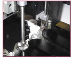
interspersed with air gaps, is also pumped through the sipper, LNF tubing and the LNF flow cell to wash away traces of the previous sample. The procedure is repeated until up to 24 samples are analyzed and processed. Sensors monitor the complete process, step by step, and shut down the system if an error occurs.
